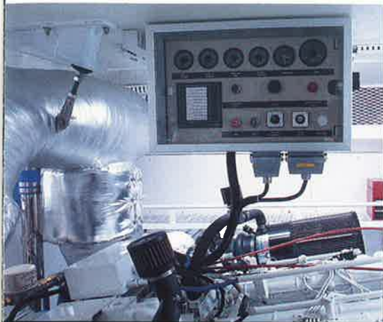
Optional Deutz-MWM TBD 616 V16 inboard diesels come with complete engine-room instrumentation to make servicing easier.
